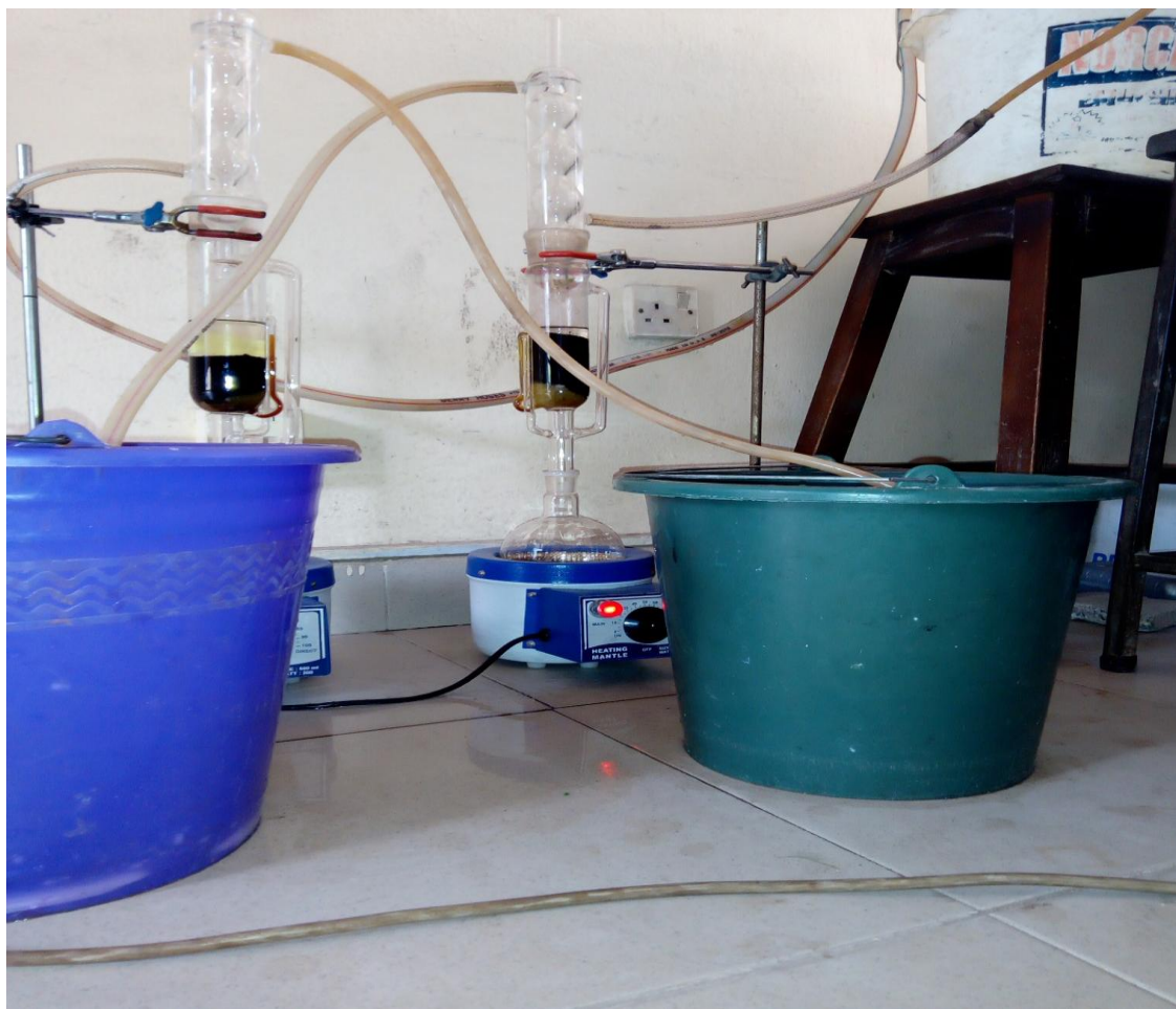
Plate 1: Image of the setup of a Soxhlet Extractor Aqueous Extractions
